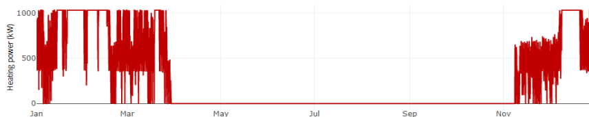
Fig. 6 Combined Heat and Power plant - Produced heating energy annually in hourly resolution
