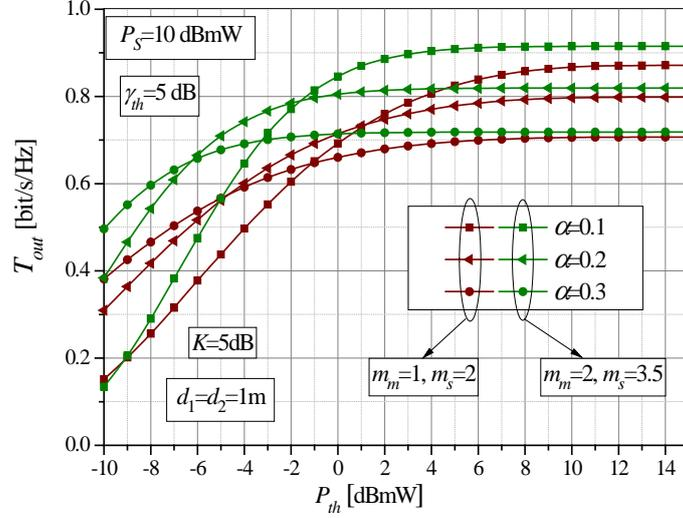
**Fig. 7** The throughput  $T_{out}$  versus threshold power, for various values of time-switching coefficient  $\alpha$  and various values of the relay-IoT channel parameters.
