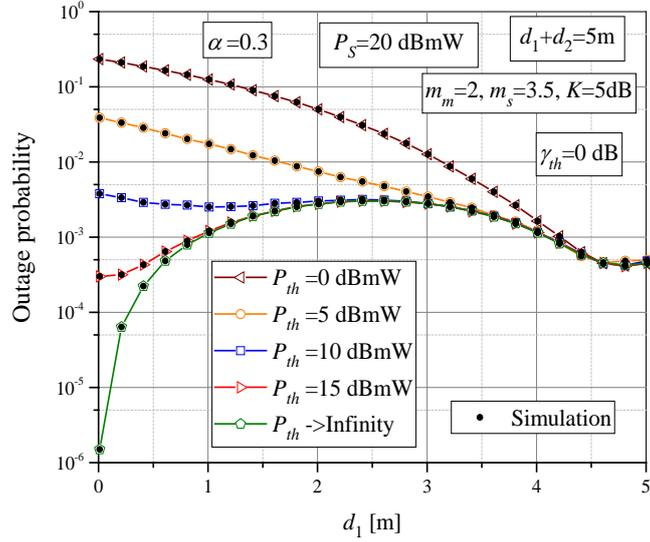
**Fig. 3** Outage probability versus source-relay node distance  $d_1$  for various values of threshold power.
