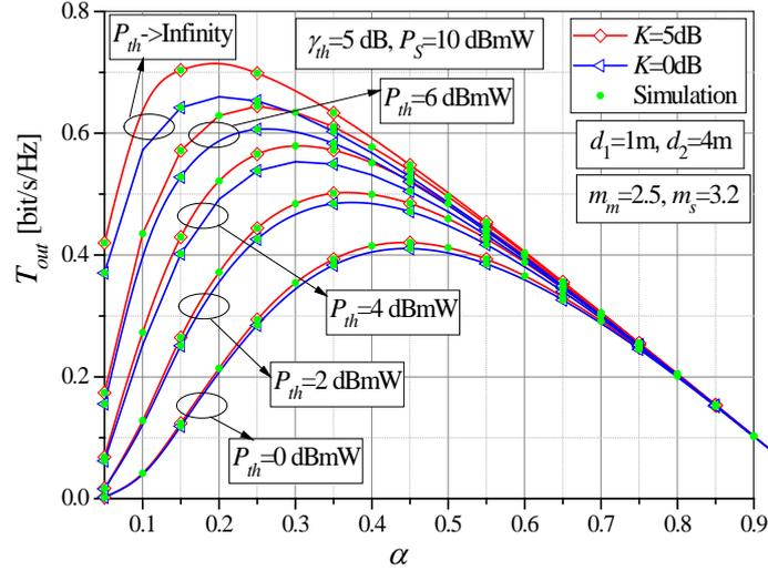
**Fig. 6** The throughput  $T_{out}$  versus time-switching coefficient  $\alpha$ , for various values of the Rician  $K$  factor and threshold power.
