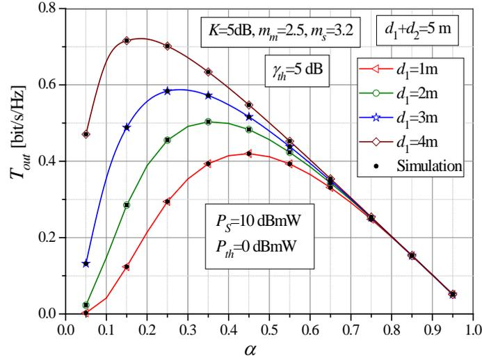
**Fig. 5** The throughput  $T_{out}$  versus time-switching coefficient for various relay distance from the source,  $d_1$ .
