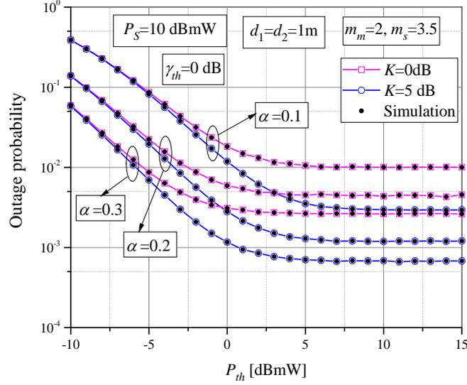
**Fig. 4** Outage probability versus threshold power for various values of the Rician  $K$  factor and time-switching coefficient.
