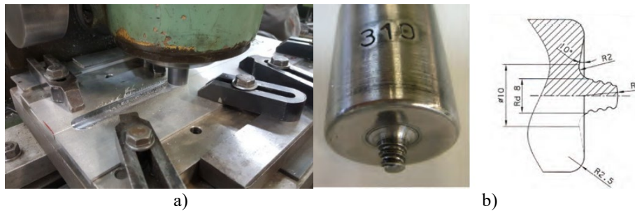
Fig. 2 Conventional Milling Machine for FSW (a) and FSW tool and tool geometry (b)
