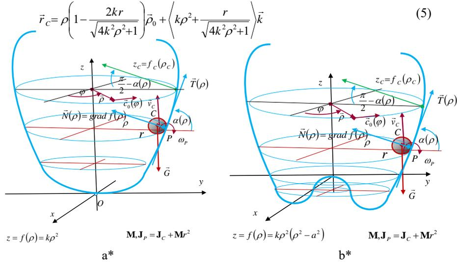
**Fig.3.** Kinematic parameters of the nonlinear dynamics of rolling a heavy, homogeneous and isotropic ball a\* on a revolving parabolic surface, and b\* on a revolving biquadratic parabolic surface: the velocity of the center of mass of the ball at the point of contact of the rolling ball and the revolving surface
