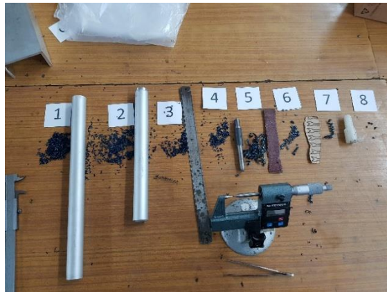
Fig. 2 Chip shapes formed under various cutting conditions
