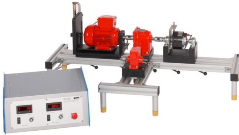
Fig. 3 GUNT AT 200 Determination of gear efficiency
