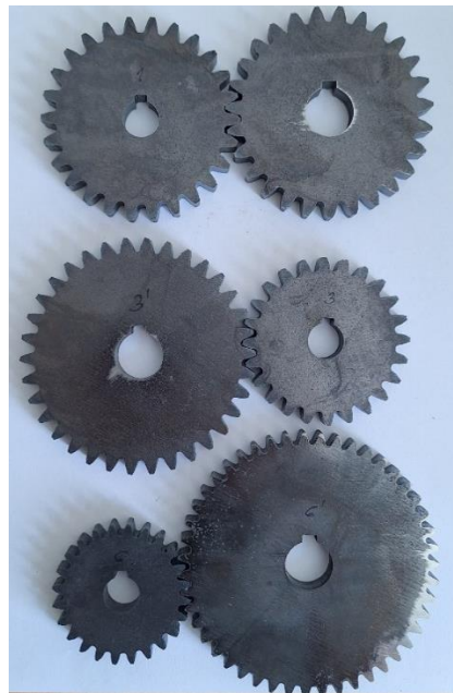
Fig. 2 Laser-cut produced spur gear pairs
