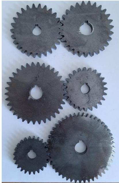
Fig. 2 Laser-cut produced spur gear pairs
