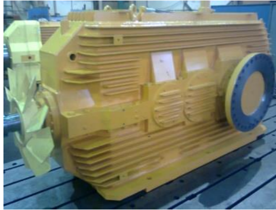
Fig. 7 Gearboxes with a fan on the proof-stand
