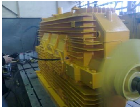
Fig. 11 Measuring vibration velocity (example)
