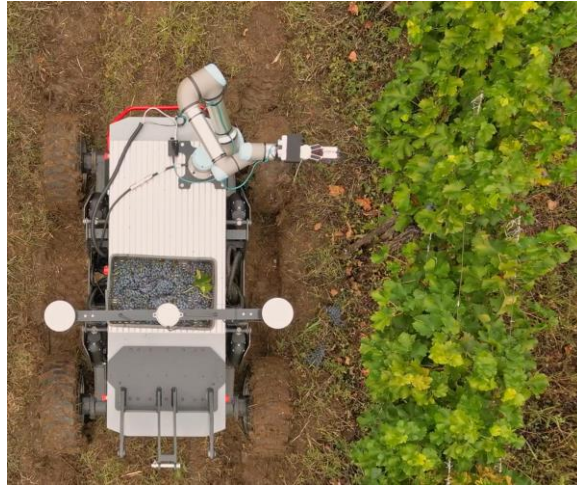
Fig.11 AgAR platform equipped with a robotic system for grape harvesting
