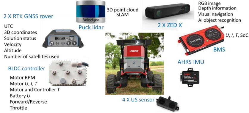
Fig. 7 AgAR sensor stack
