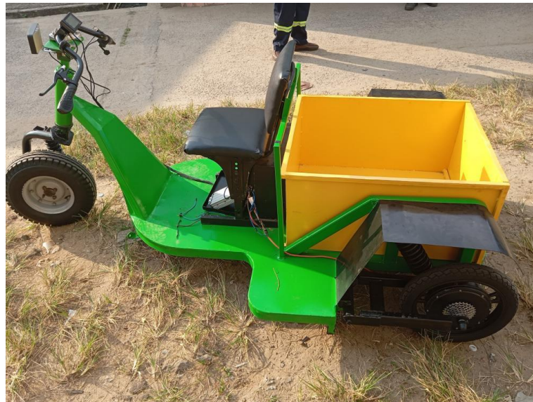
Fig. 9 Fully Assembled Product of the Battery Powered Tricycle
