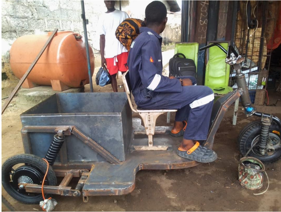
Fig. 8 Photo of the first tricycle relevant parts assembling ready for mechanical testing
