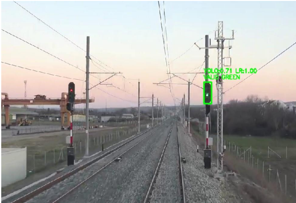
Fig. 4 Preliminary integration of YOLO detection with HOG + Logistic Regression validation in real railway video frames
