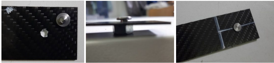
Fig. 3 Inserting a steel element in CFRP
