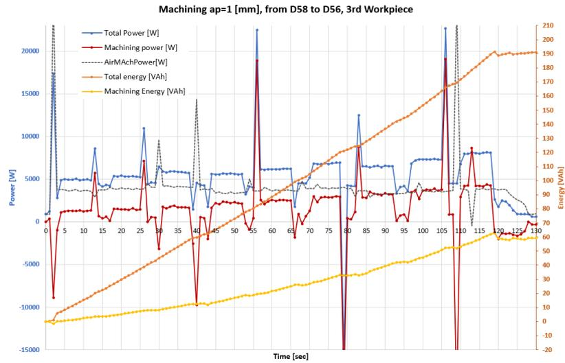
**Fig. 7** Differential diagram of engaged power and energy consumption for the case of  $a_p=1$  [mm] and  $D_6=58$  [mm] (3<sup>rd</sup> workpiece)
