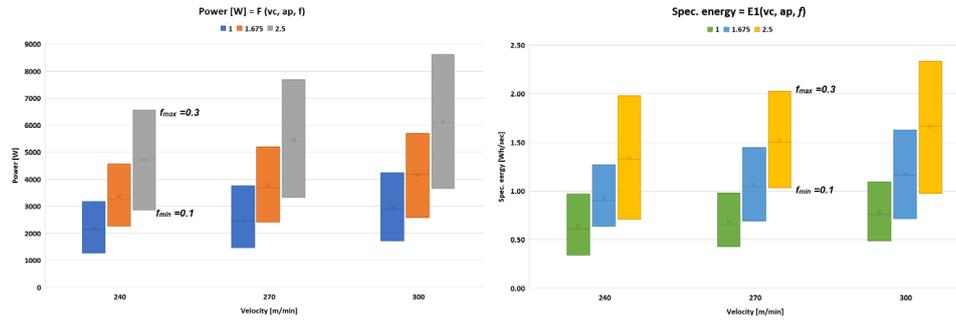
Fig. 9 Effect of feed rate on P and  $E_{\text{spec}}$
