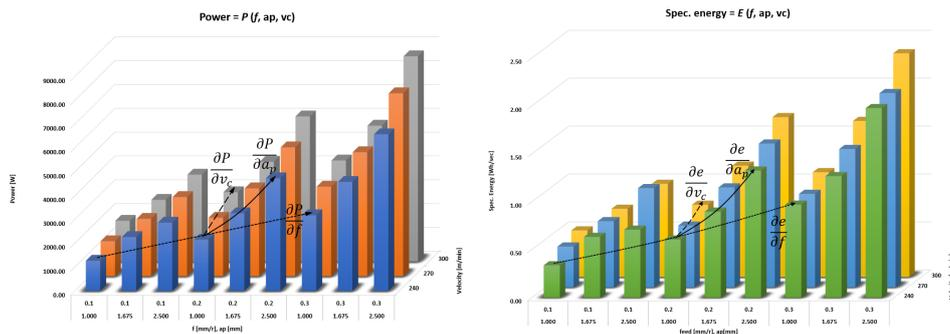
**Fig. 8** Change in engaged power and specific energy consumption with respect to the cutting parameters change
