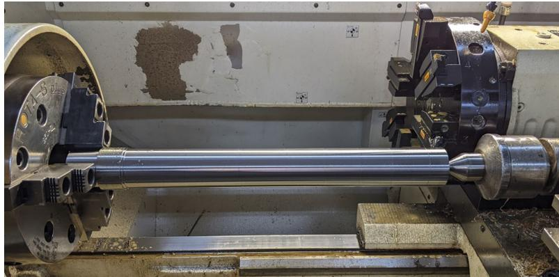
**Fig. 1** Setup of the workpiece in the lathe.
