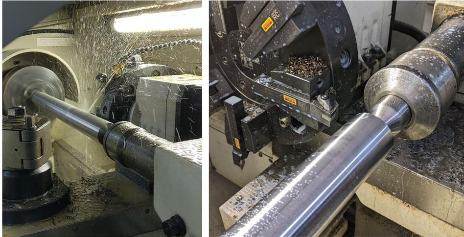
**Fig. 5** Machining in wet conditions
