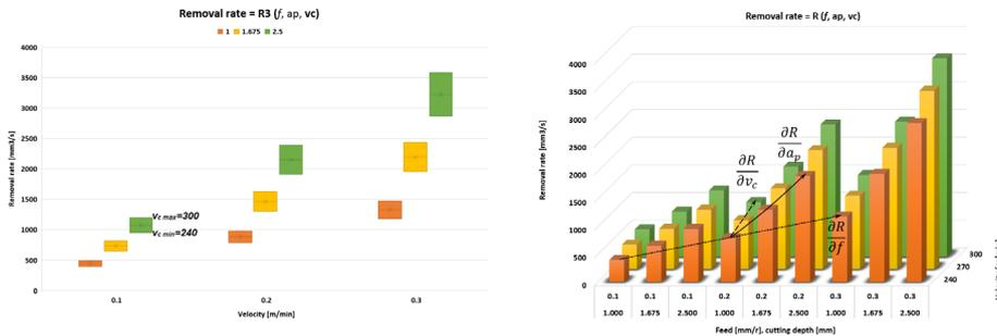
**Fig. 13** Effect of cutting speed on material removal rate (left) and change in material removal rate with respect to cutting parameters change (right)
