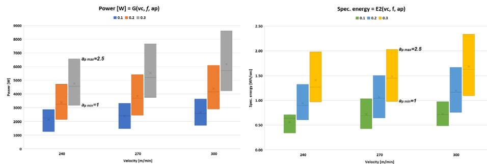
Fig. 10 Effect of depth cut on P and  $E_{\text{spec}}$
