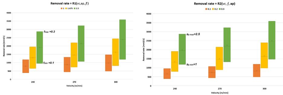
**Fig. 12** Effect of feed rate on material removal rate (left) and effect of depth of cut on material removal rate (right)
