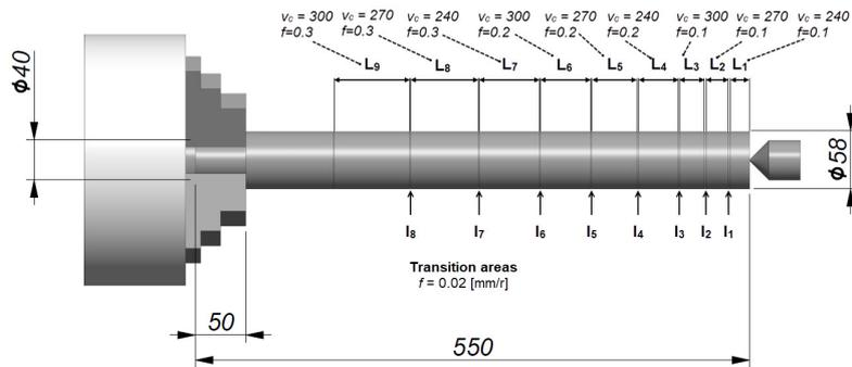
Fig. 4 The machining segments' disposition along the workpiece for the experiment
