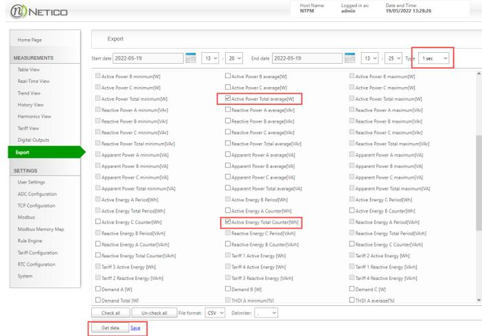
**Fig. 3** Selection of the values to be recorded from the control panel of the NTPM Sensor: Active Energy Total [Wh] Active Power Total Average [W]
