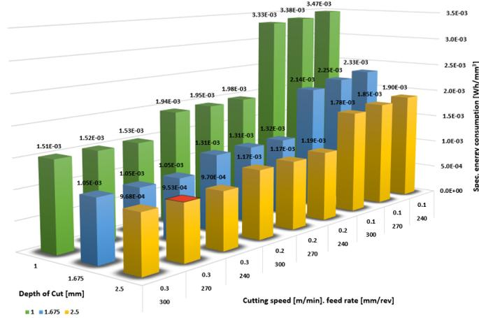
Fig. 15 The specific energy consumption with regard to material volume removal rate.
