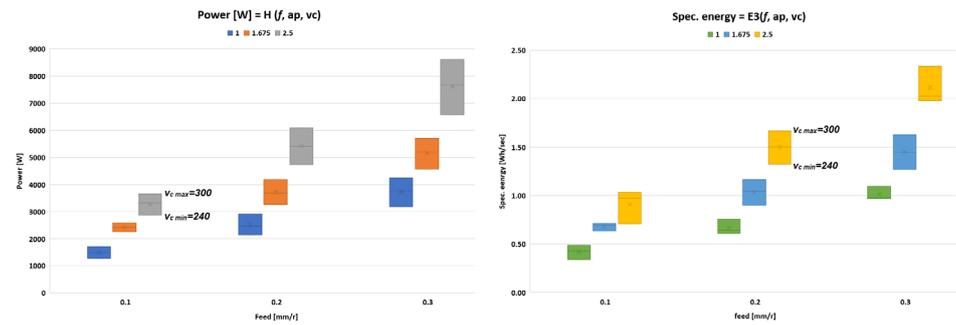
Fig. 11 Effect of cutting speed on P and  $E_{\text{spec}}$
