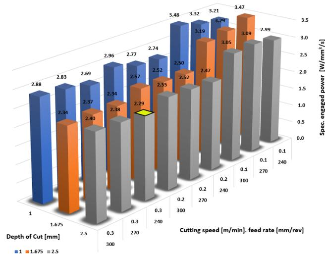
Fig. 14 The engaged power with regard to material volume removal rate.
