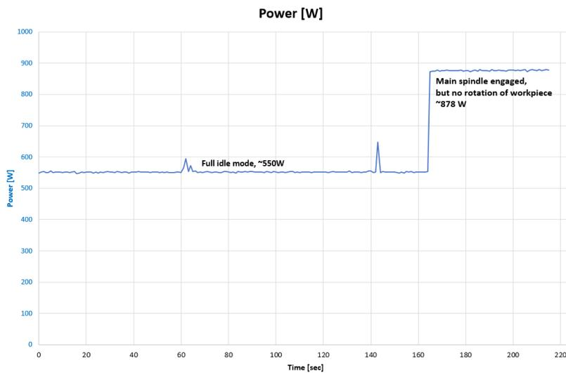
**Fig. 6** Engaged power in idle mode
