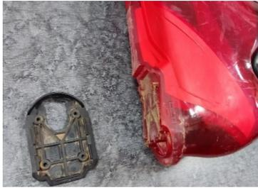
a) Broken thread part of a ski shoe heel
