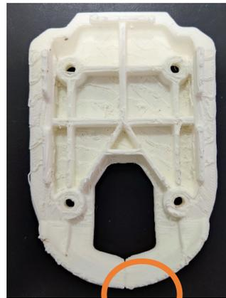
d) Printed model with visible defect
