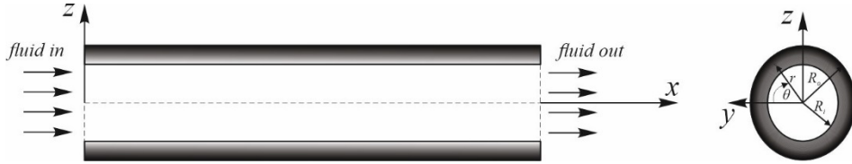
Fig. 1 Geometry and coordinates of FG nanotube model
