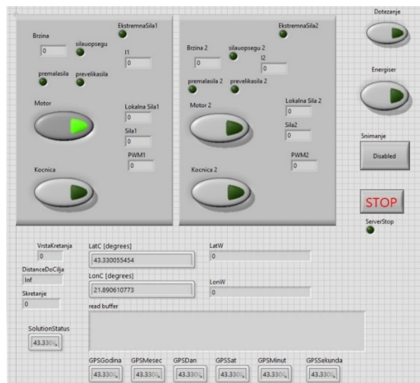
Fig. 5 Front panel in LabVIEW of the developed data acquisition system
