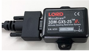
Fig. 8 3DM-GX5-25 Lord Microstrain IMU
