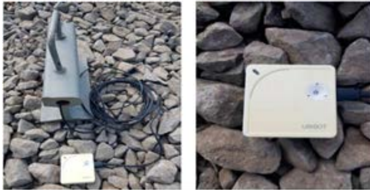
Fig. 5 Measuring station Tszyn WS1 WIFI with rail type S49 (49E1) [9]
