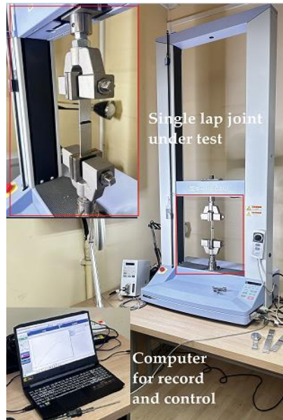
Fig. 3 Setup for the shear test with a single lap joint on Shimadzu AGS-X
