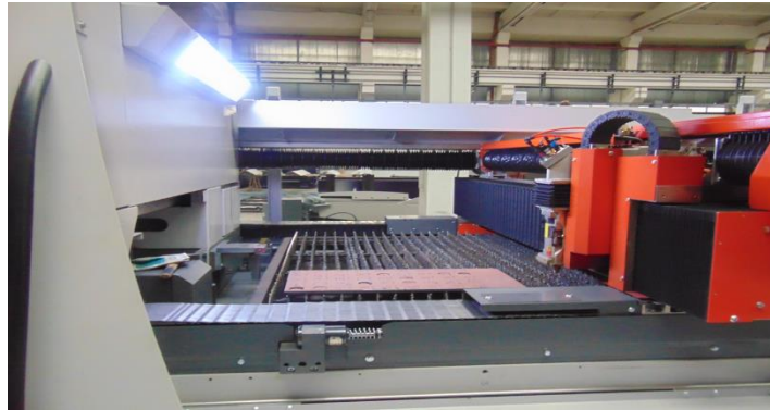
Fig. 2 Bystronic ByAutonom 3015 installation
