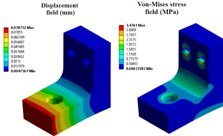
Fig. 4 Result of FEA of L-bracket with solid internal structure
