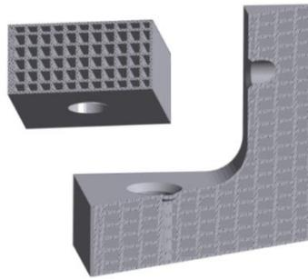
**Fig. 11** Cross-sections of the bracket with classical infill
