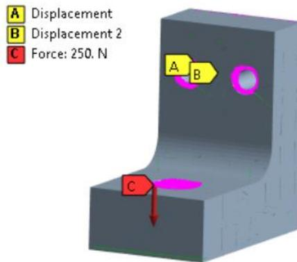
Fig. 9 Optimized L-bracket boundary conditions
