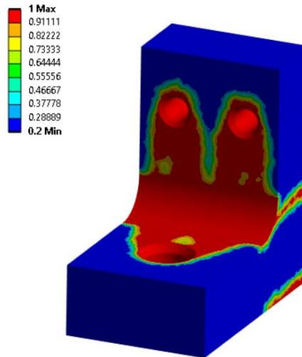
**Fig. 7** The first result of structural optimization – lattice density distribution
