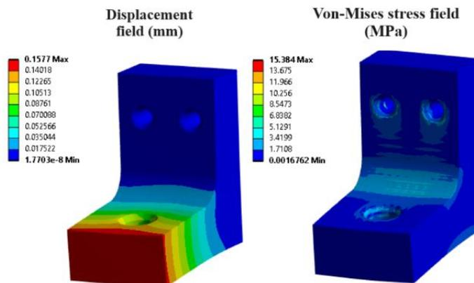
**Fig. 12** Result of FEA of L-bracket with classical infill
