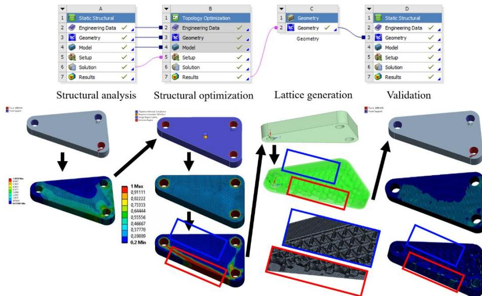
Fig. 5 Lattice optimization workflow.
