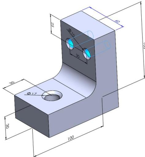
**Fig. 2** CAD model of L-bracket with dimensions (mm)
