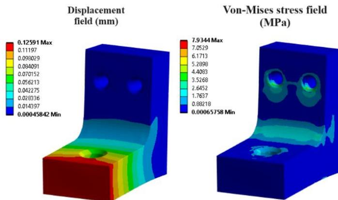
Fig. 10 Result of FEA of optimized L-bracket
