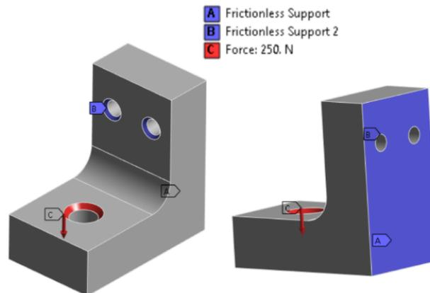
**Fig. 3** Loads and boundary conditions imposed on the FE model of L-bracket
