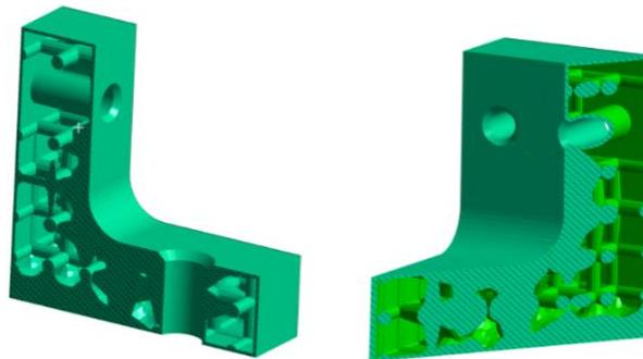
**Fig. 8** Cross-sections of the optimized bracket with lattice infill
