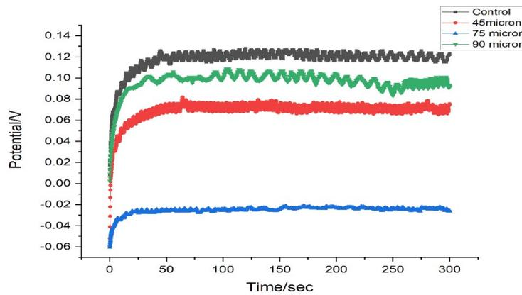
Fig.3. Open circuit potential plots of brake pad samples in stagnant water
