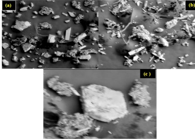
**Fig.6.** SEM microstructure of developed brake pad with (a) 45  $\mu\text{m}$ , (b) 75  $\mu\text{m}$  and (c) 90  $\mu\text{m}$  snail shell particles.
