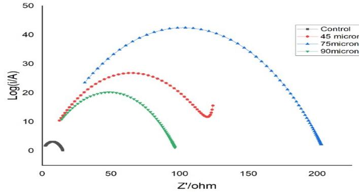
**Fig. 5.** Nyquist plots for developed brake pad in stagnant water
