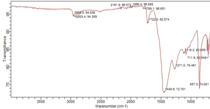
Fig. 2. FTIR spectrum of the developed brake pad.
