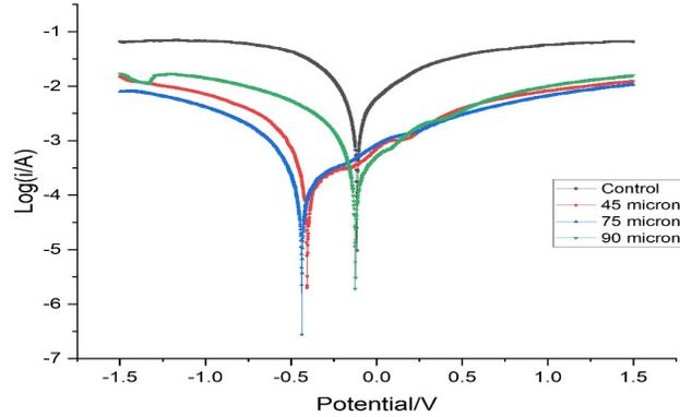
**Fig.4.** Tafel plots of developed brake pad at different grain size in stagnant water
